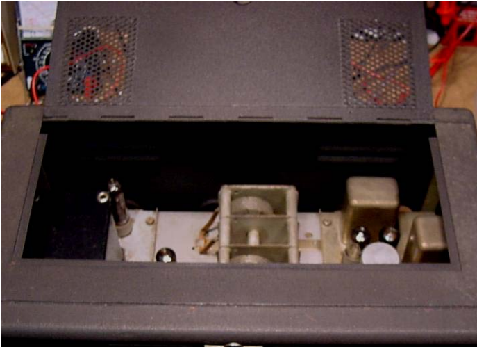
Above: Lid open – the picture tube is hidden below the upper (tuner) sub-chassis visible in this photo
